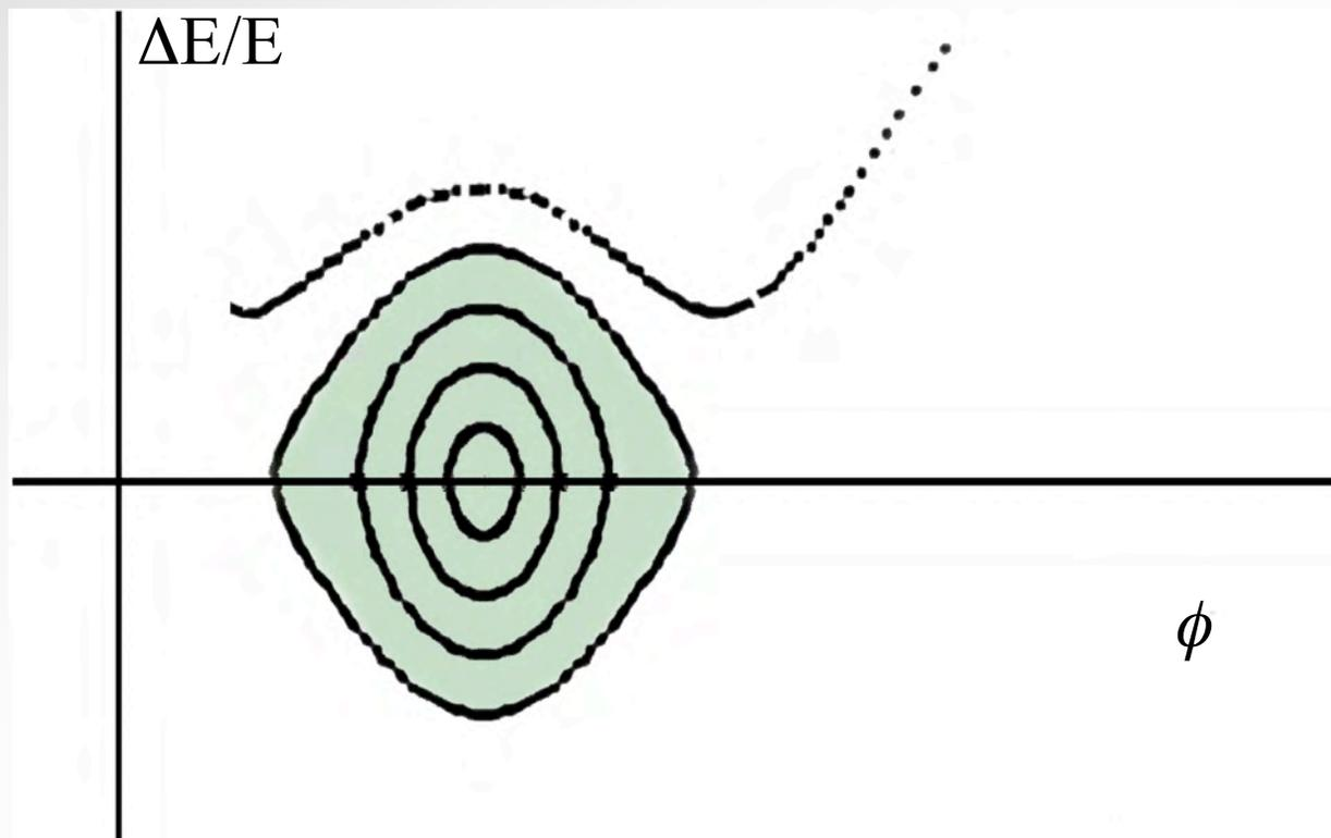
*Solving the difference equations will show if there are areas of stability in the  $(\Delta E/E, \phi)$  longitudinal phase space of the beam*
